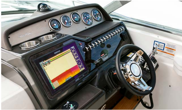
The well-designed, tiered helm station features standard Digital Dash with Mercury® VesselView Link Data with Simrad G09 (9") Touchscreen Display & Chartplotter.
